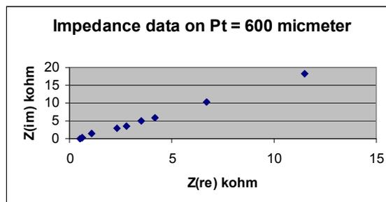
Fig. 1:  $Z(re) - Z(im)$  plot for platinum electrode of radius = 600  $\mu m$  (0.1M TBAP, MeCN solvent).
