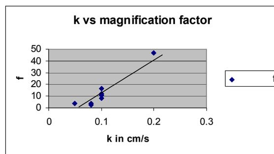
Fig. 7: Standard heterogeneous electron transfer rate constant  $k_0$  vs  $f_m$  (magnification factor). The correlation factor  $r^2 = 0.92$ .
