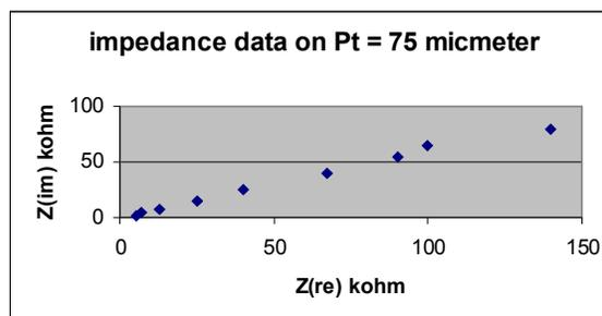
Fig. 3:  $Z(re) - Z(im)$  plot for platinum electrode of radius = 75  $\mu m$  (0.1M TBAP, MeCN solvent).
