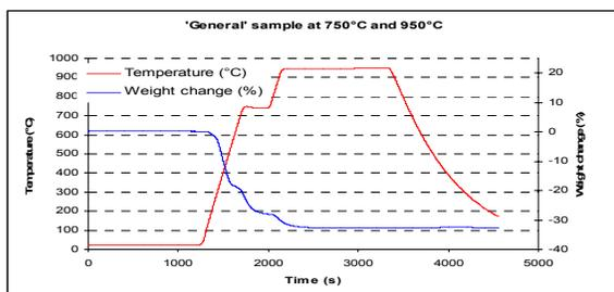
Fig. 8: Thermo-gravimetric analysis of mixed waste at 750 and 950 °C.
