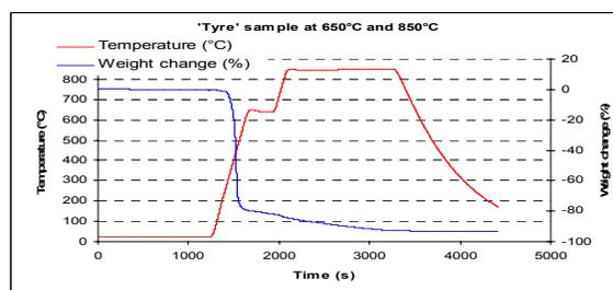
Fig. 3: Thermo-gravimetric analysis of tyre waste at 650 and 850 °C.
