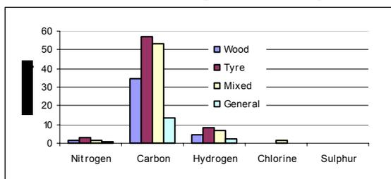
Fig. 2: Ultimate analysis results of auto shredder waste streams and wood.
