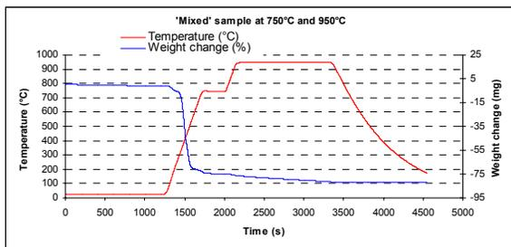
Fig. 6: Thermo-gravimetric analysis of mixed waste at 750 and 950 °C.
