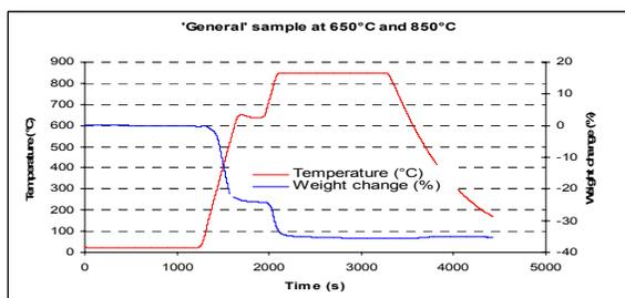
Fig. 7: Thermo-gravimetric analysis of general waste at 650 and 850 °C.
