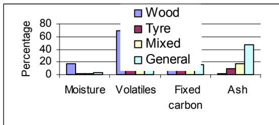
Fig. 1: Comparison of proximate analysis of auto shredder waste streams with wood.
