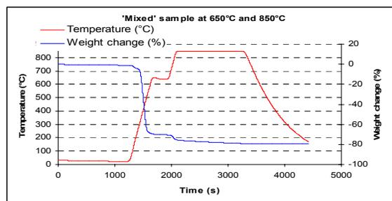
Fig. 5: Thermo-gravimetric analysis of mixed waste at 650 and 850 °C.
