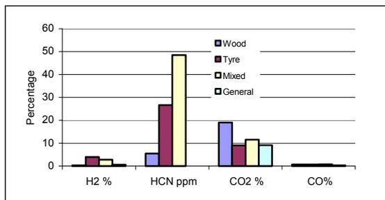
Fig. 10: Comparison of gas analysis results for auto shredder waste and wood.
