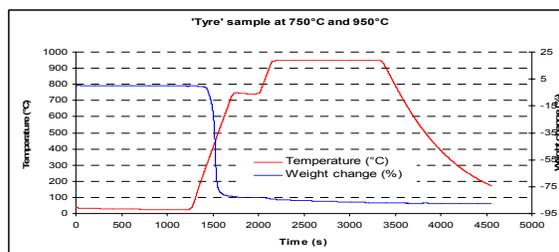
Fig. 4: Thermo-gravimetric analysis of tyre waste at 750 and 950 °C.
