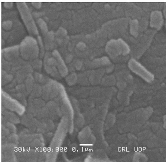
Fig. 1: Scanning electron micrograph of MnO<sub>2</sub> with 100,000 magnification.
