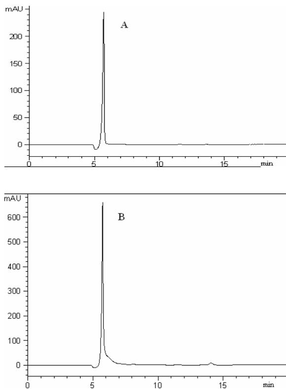
Fig.3: HPLC chromatograms of (A) standard glucuronic acid (1.0 mg/ml), and (B) acid hydrolysed chondroitin sulphate from fish heads (3.0 mg/ml).
