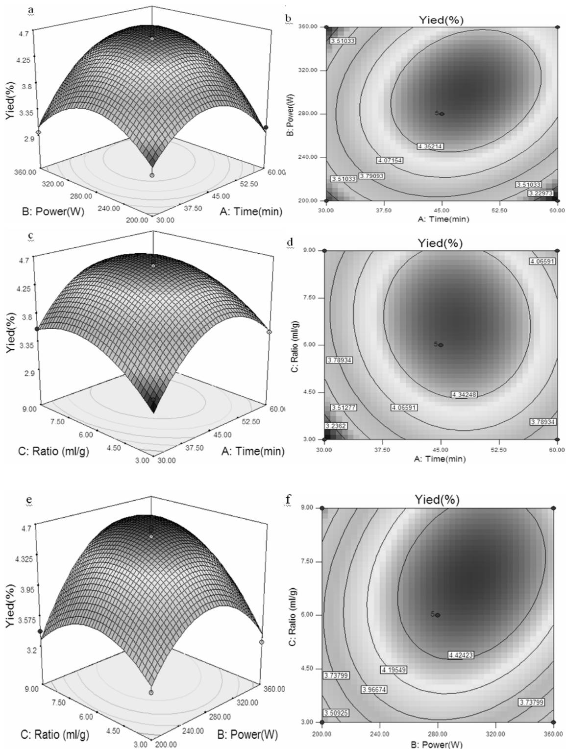
Fig.2: Response surface plots (a, c and e) and contour plots (b, d and f) showing the effects of ultrasonic time, ultrasonic power, solvent/material ratio and their mutual effects on CS.
