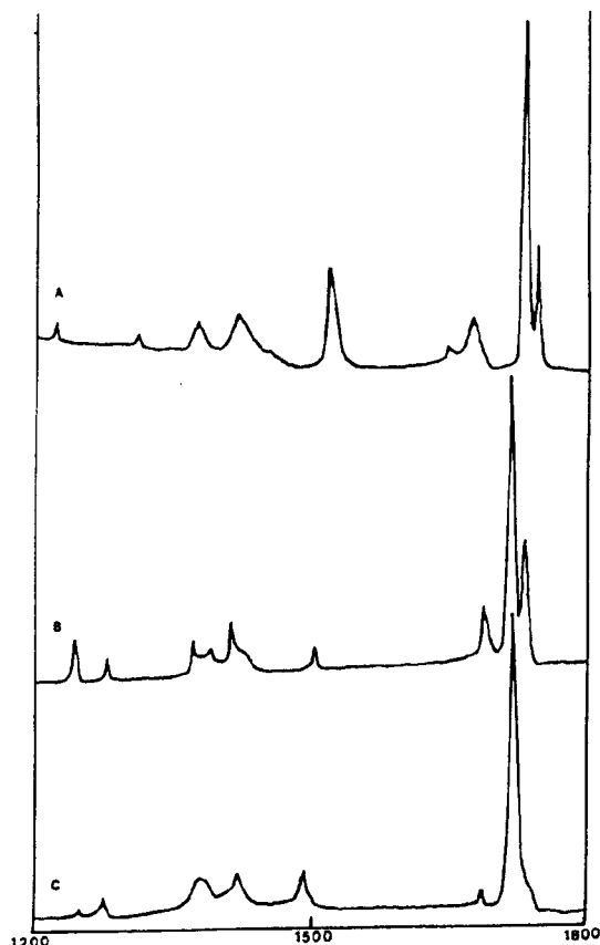
Fig.2: Raman Spectra of: A) Diacetamide (trans-); B) \text{Co}[(\text{DA})_4(\text{H}_2\text{O})_2]\text{Br}_2 ; C) \text{Co}[(\text{DA})_2(\text{H}_2\text{O})_2]\text{Br}_2 ;
