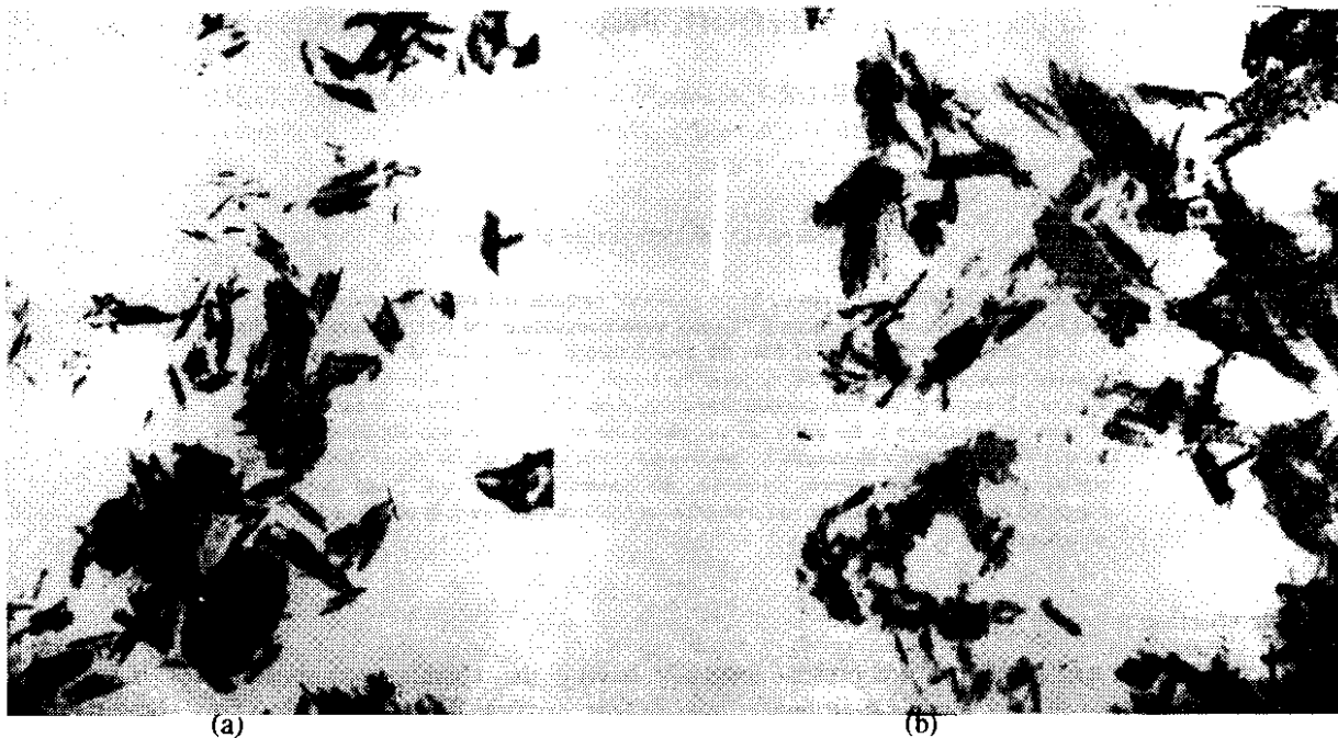
Fig. 1: Transmission electron micrographs of \alpha -FeOOH particles: (a) Sample-1, (b) Sample-2. Magnification, 70,000 x.
