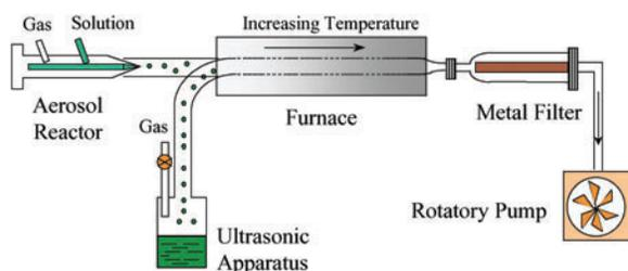
Fig. 7: Schematic demonstration of the spray pyrolysis device, used for the synthesis of MNPs.
