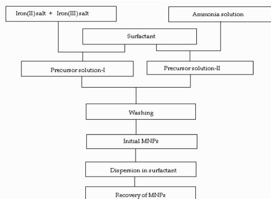
Fig. 4: Procedure for the synthesis of MNPs by chemical coprecipitation method.
