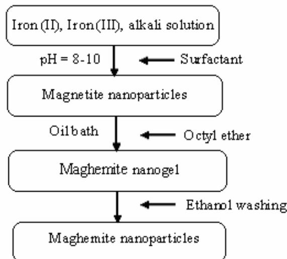
Fig. 6: Scheme for the synthesis of MNPs via sol-gel method.
