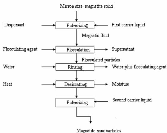
Fig. 3: Pulverization of bulk magnetite in the presence of solvent and surfactants.
