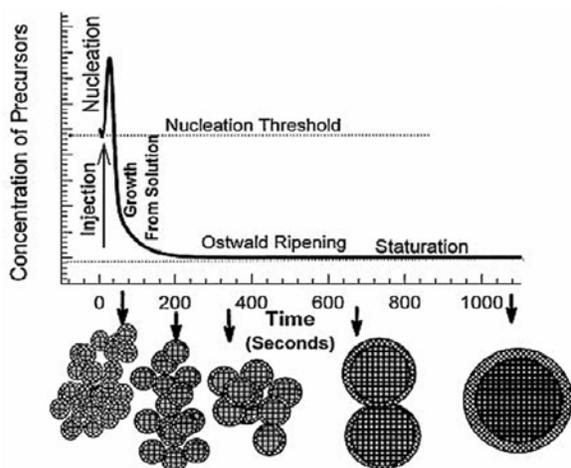
Fig. 2: Diagram depicting the stages of nucleation and growth for the synthesis of monodispersed nanoparticles based on the work of LaMer and Dinegar.
