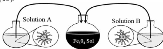
Fig. 5: W/O microemulsion method for producing MNPs in nonpolar solvents (solution A and solution B contains Iron(II)/Iron(III) and ammonia solutions respectively).
