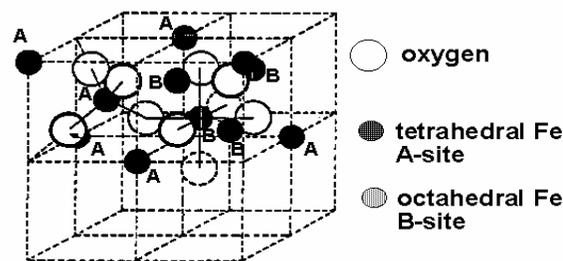
Fig. 1: Inverse spinel crystal structure of magnetite.
