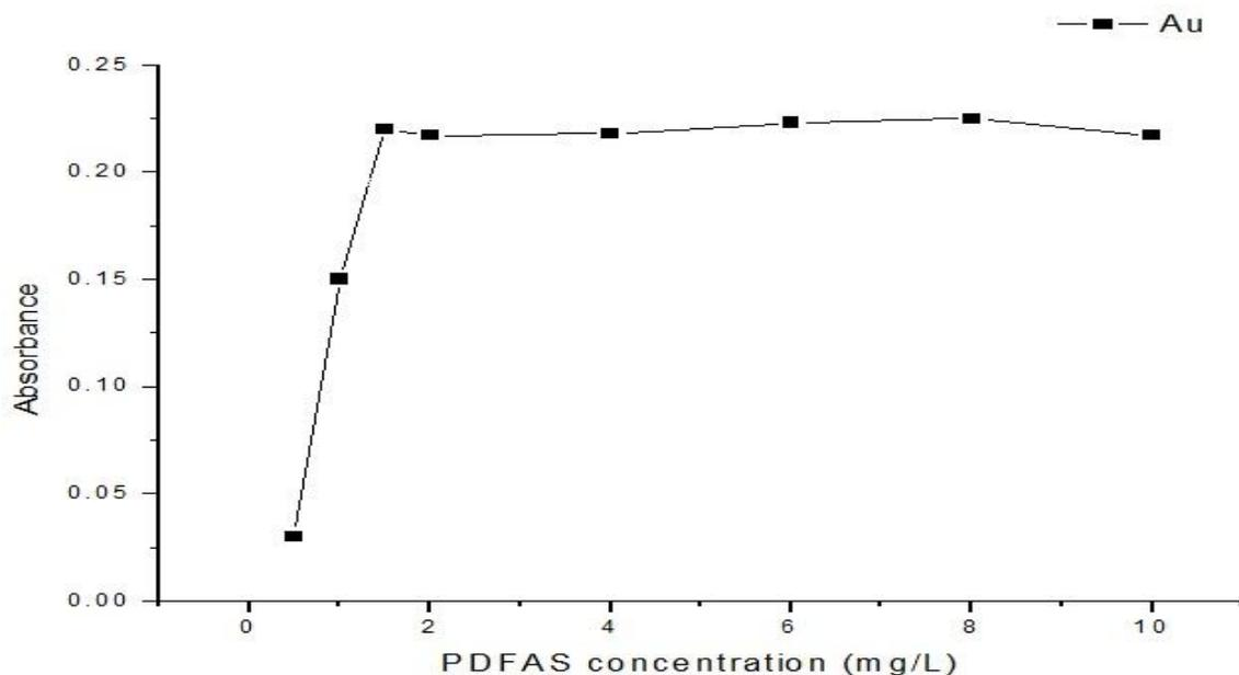
Fig. 4: Effect of the PDFAS concentration on the cloud point extraction of Au. Other experimental conditions were the concentration of TMN-6 was 5% (v/v), the temperature was 45 °C, the equilibrium time was 30 min, pH=4, respectively.
