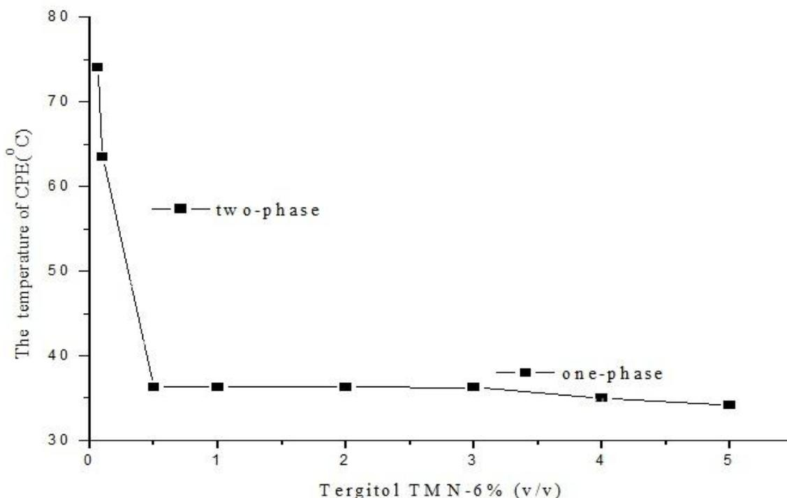
Fig. 1: Cloud point of TMN-6 solution as a function of surfactant concentration. Other experimental conditions were the concentration of TMN-6 was 5% (v/v) and the concentration of PDFAS was  $0.1 \text{ g/L}$ , the temperature was  $45 \text{ }^{\circ}\text{C}$ , the equilibrium time was 30 min,  $\text{pH}=4$ , respectively.
