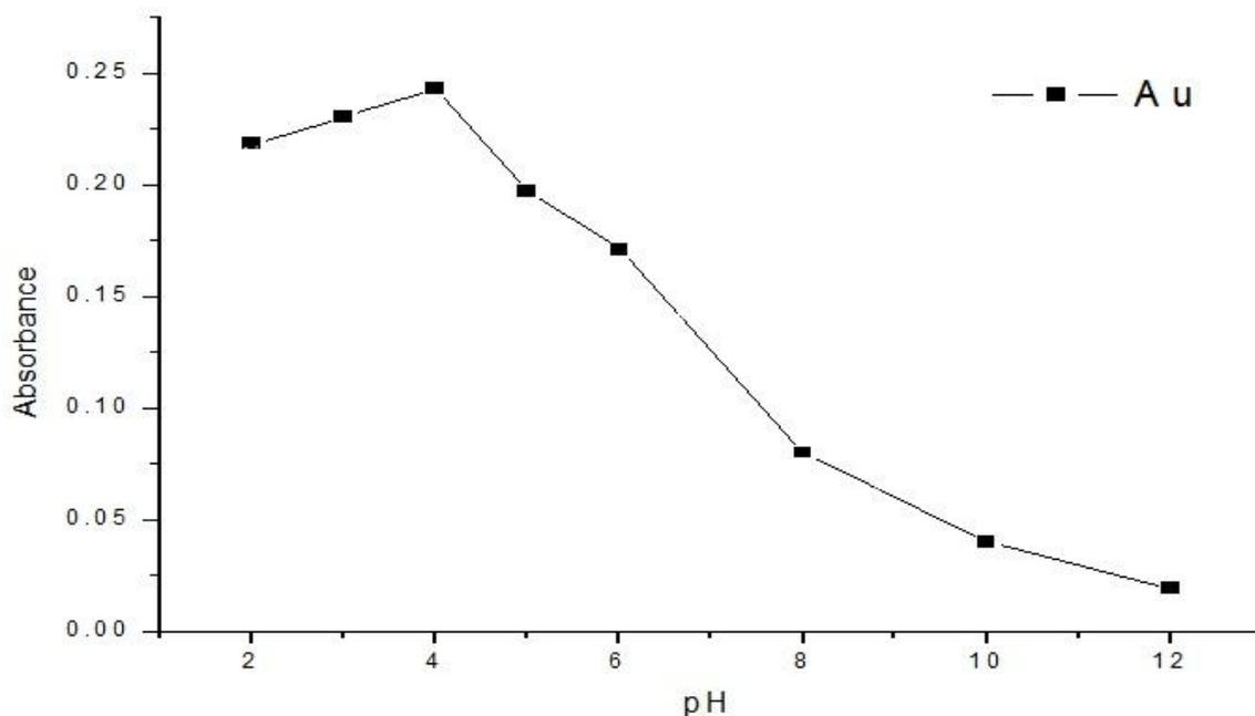
Fig. 2: Effect of pH on the cloud point extraction of Au. Other experimental conditions were the concentration of TMN-6 was 5% (v/v) and the concentration of PDFAS was 0.1g/L, the temperature was 45 °C, the equilibrium time was 30 min, respectively.
