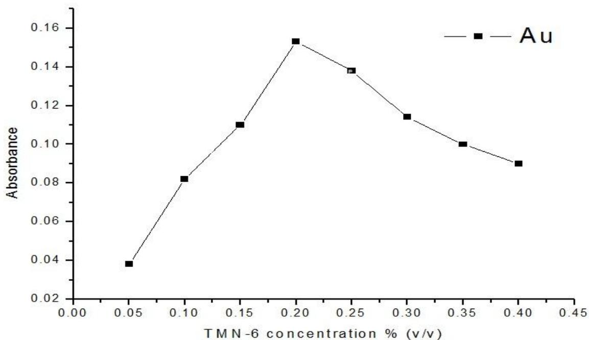
Fig. 3: Effect of Tergitol TMN-6 concentration on the cloud point extraction of Au. Other experimental conditions are concentration of PDFAS was 0.1g/L; equilibrium temperature: 45 °C; equilibrium time: 30 min; pH=4. Other experimental conditions were the concentration of PDFAS was 0.1g/L, the temperature was 45 °C, the equilibrium time was 30 min, pH=4, respectively.
