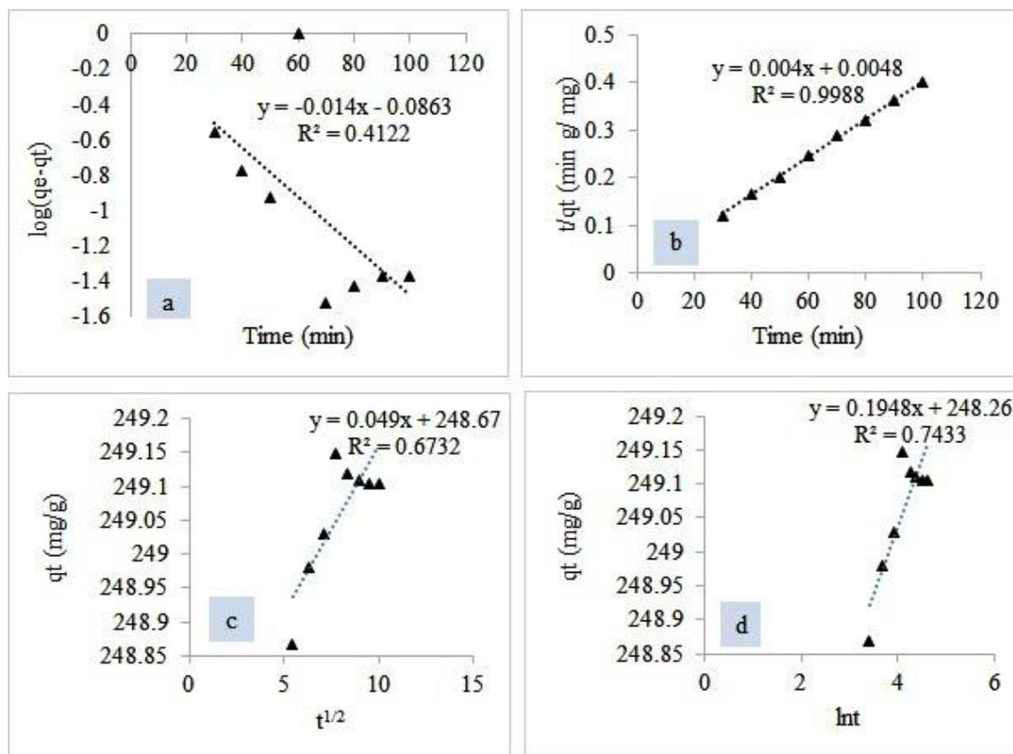
Fig 7: Pseudo-first order kinetics plot (a), Pseudo-second order kinetics plot (b), Intraparticle diffusion (c) and Elovich model plot (d) for the adsorption of FPE on SMFE (Ci=1000 mg L<sup>-1</sup>, pH 6.0, T=298K).
