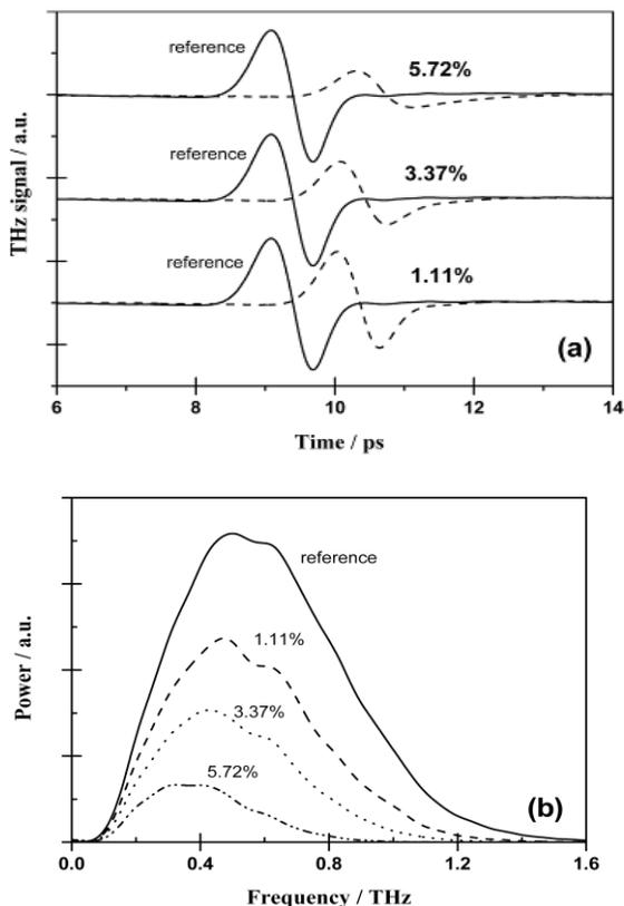
Fig. 1: Time-domain wave forms (a) and frequency-domain spectra (b) for the reference and composites filled with thin MWNTs at different concentration.
