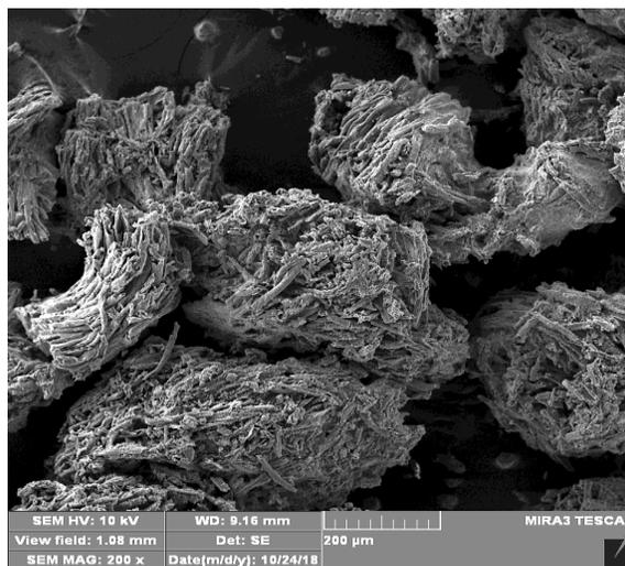
Fig. 4: SEM micrograph of the used adsorbent.
