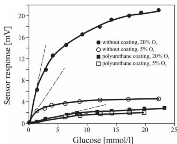
Fig. 4: Calibration curves of sensor at different oxygen concentrations without coating (● 20%, ○ 5% oxygen) and with polyurethane coating (■ 20%, □ 5% oxygen), respectively.
