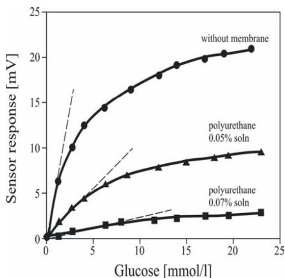
Fig. 3: Sensor characteristics without an outer diffusion control coating ( $\bullet$ ) and with polyurethane coating, casted from 0.05% ( $\blacktriangle$ ) – 0.07% ( $\blacksquare$ ) solution.
