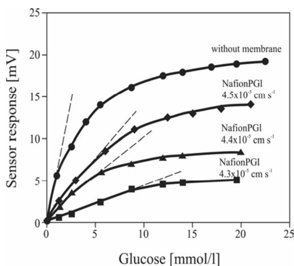
Fig. 2: Sensor characteristics without an outer controlling membrane ( $\bullet$ ) and with Nafion membranes of different glucose permeabilities ( $\blacklozenge$  PGI =  $4.5 \times 10^{-5} \text{ cm s}^{-1}$ ,  $\blacktriangle$  PGI =  $4.4 \times 10^{-5} \text{ cm s}^{-1}$ ,  $\blacksquare$  PGI =  $4.3 \times 10^{-5} \text{ cm s}^{-1}$ ).
