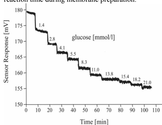
Fig. 1: Sensor response of the amperometric electrode towards different glucose concentrations.
