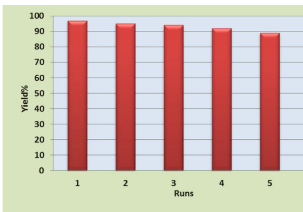
Fig. 6: Reusability of \text{Fe}_3\text{O}_4@\text{TiO}_2\text{-H}_5\text{IO}_6 in the reaction of benzaldehyde, o -phenylenediamine, and dimedone.
