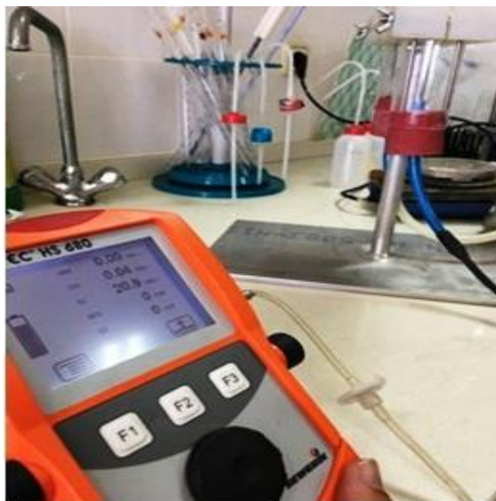
Fig. 9: Gas measurement at the end of the experiment.
