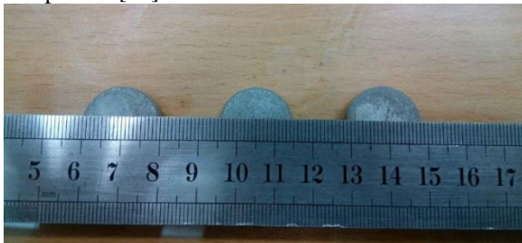
Fig. 1: Showing prepared composites samples after sintering and Heat treatment. It can be seen that only a slight variation in diameter is observed after sintering and the samples have diameters around 18-19 mm contrary to 20 mm initial diameter.
