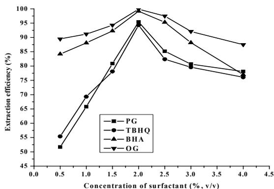
Fig. 5: Effect of mixed surfactant concentration of NP-7 + NP-9 on the extraction efficiency
