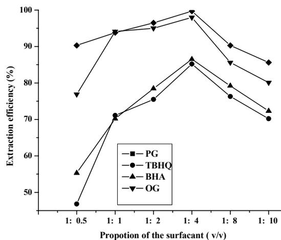
Fig. 4: Effect of mixing proportion of NP-7 and NP-9 on the extraction efficiency. Other experimental conditions are concentration of surfactant: 2.0% (v/v); equilibrium temperature: 55 °C; equilibrium time: 40 min
