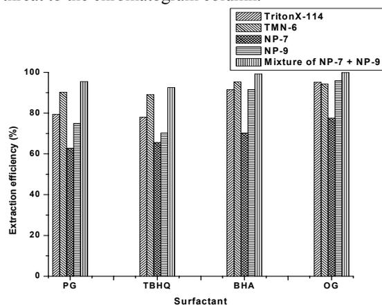
Fig. 2: Effect of different kinds of surfactants on the extraction efficiency of the SPAs spiked in cake: concentrations of Triton X-114, Tergitol TMN-6, NP-7 or NP-9 are 2.0% (v/v), respectively
