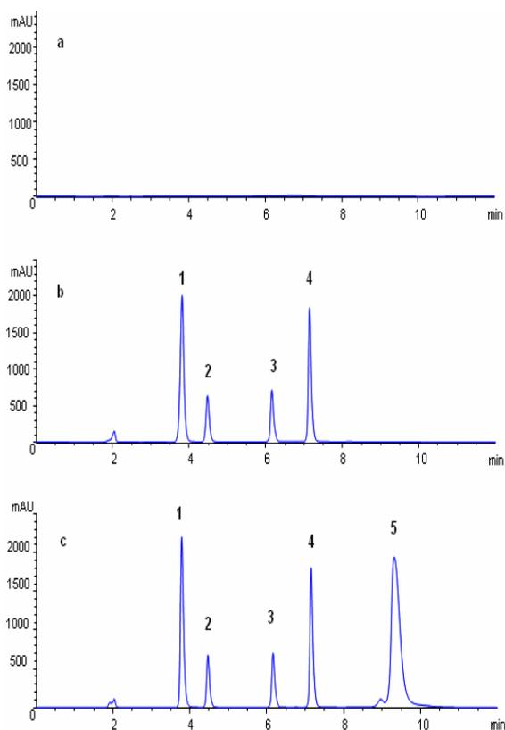
Fig. 3: HPLC–UV chromatograms: a blank cake, b standard ( $600 \mu\text{g mL}^{-1}$ ) and c cake spiked with SPAs ( $600 \mu\text{g mL}^{-1}$ , peaks were obtained by dilute the surfactant-rich phase from 0.3mL to 0.6mL). Peak nr: (1) PG, (2) TBHQ, (3) BHA, (4) OG, (5) NP-7 + NP-9. HPLC conditions-gradient separation using methanol and 0.1 % (v/v) acetic acid; injection volume 10  $\mu\text{L}$ ; flow rate 1  $\text{mL min}^{-1}$ ; wavelength 280 nm
