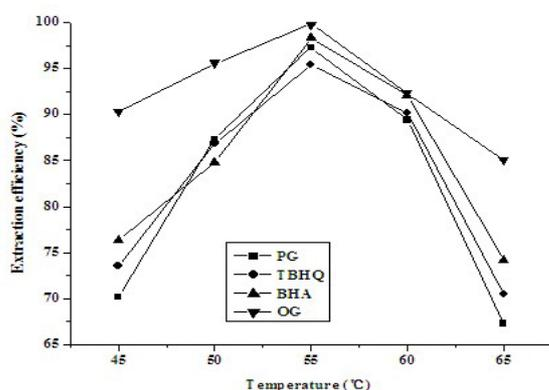
Fig. 6: Effect of the equilibrium temperature on the extraction efficiency.
