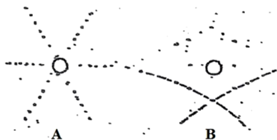
Fig. 11: Laue back-reflection photographs: (A) with x-ray beam perpendicular to the basal plane (0001); (B) with x-ray beam perpendicular to a prism plane (1120). Dashed lines on the photograph are drawn to show that the back-reflection spots lie on hyperbolas. [7]
