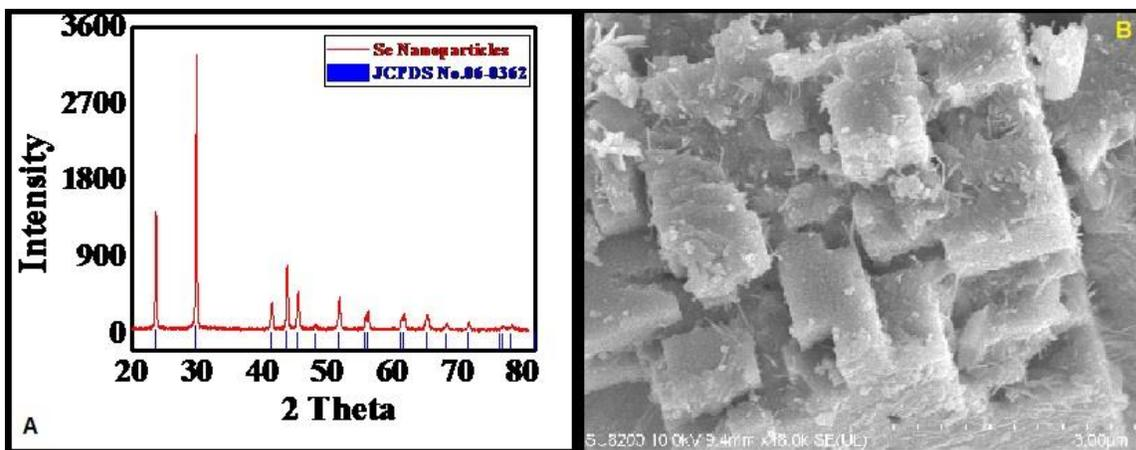
Fig. 1: (A) X ray diffraction (XRD) pattern and (B) Scanning electron micrograph (SEM) of the Selenium nanoparticles synthesized by organic acid induced method during present study.
