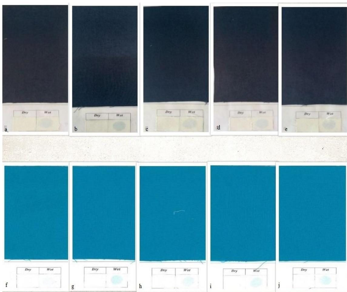
Fig. 1: Resin treatment on colorfastness to crocking of dyed cotton fabric (a) untreated sample (b) sample treated with Fixapret ECO 50g/L (c) sample treated with Fixapret ECO 100g/L (d) sample treated with Alkakit WFR 50g/L (e) sample treated with Alkakit WFR 100g/L (f) untreated sample (g) sample treated with Fixapret ECO 50g/L (h) sample treated with Fixapret ECO 100g/L (i) sample treated with Alkakit WFR 50g/L (j) sample treated with Alkakit WFR 100g/L.
