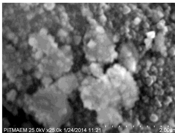
Fig. 5: SEM micrograph of composite NCS-1.
