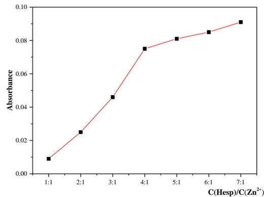
Fig. 4: Method of molar ratios: mixture of  $1.00 \times 10^{-4}$  mol/L  $\text{ZnCl}_2$  and hesperidin (ranging from  $1.00 \times 10^{-4}$  to  $7.00 \times 10^{-4}$  mol/L), blank is hesperidin, as in mixtures.  $\lambda=369$  nm.
