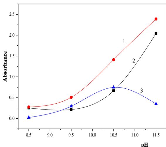
Fig. 7: Dependence of absorbance on pH at  $\lambda = 369$  nm: (curve 1)  $1.00 \times 10^{-3}$  mol/L hesperidin, blank is methanol; (curve 2) mixture of  $5.00 \times 10^{-5}$  mol/L  $ZnCl_2$  and  $1.00 \times 10^{-3}$  mol/L hesperidin, blank is 70% (v/v) methanol; (curve 3)  $\Delta A = f(pH)$ .
