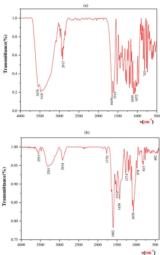
Fig. 6: IR spectra of hesperidin (a) and the Zinc(II)-hesperidin complex (b).
