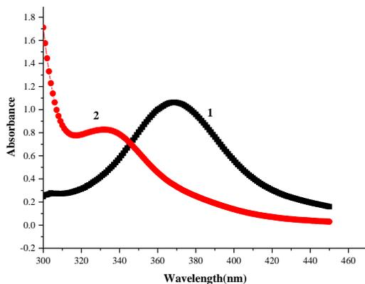
Fig. 3: UV spectra. Curve 1: mixture of  $1.00 \times 10^{-5}$  mol/L  $\text{ZnCl}_2$  and  $4.00 \times 10^{-5}$  mol/L hesperidin, blank is  $4.00 \times 10^{-5}$  mol/L hesperidin; Curve 2:  $4.00 \times 10^{-5}$  mol/L hesperidin, blank is 70% (v/v) methanol.
