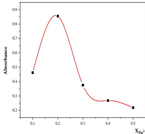
Fig. 5: Method of continual variations of equimolar solutions:  $C_{\text{Zn}^{2+}}$  plus  $C_{\text{hesp}}$  makes  $1.00 \times 10^{-3}$  mol/L, Blank is hesperidin as in mixtures,  $\lambda=369$  nm.
