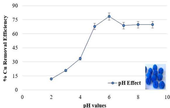
Fig. 3: Effect of pH on removal of  $\text{Cu}^{2+}$  by Hi-DBB ( $\text{Cu}^{2+}$  initial: 100 mg/L, Hi-DBB dose: 2 g, pH: 6.23, 25 °C).
