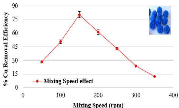
Fig. 4: Effect of mixing speed on removal of  $\text{Cu}^{2+}$  by Hi-DBB ( $\text{Cu}^{2+}$  initial: 100 mg/L, Hi-DBB dose: 2 g, pH: 6.23, 25 °C).
