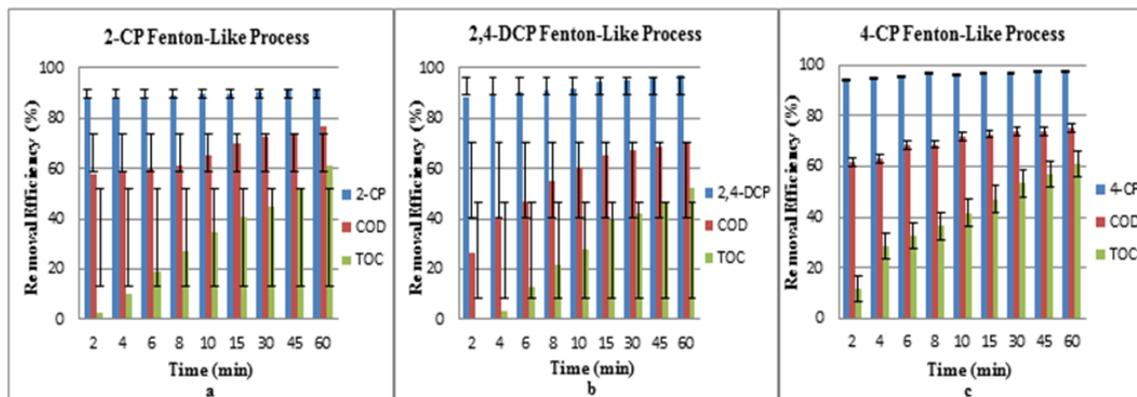
Fig. 4: Removal efficiencies with Fenton-Like process (optimum conditions).
