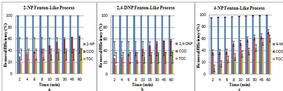
Fig. 5: Removal efficiencies with Fenton-Like process (optimum conditions).
