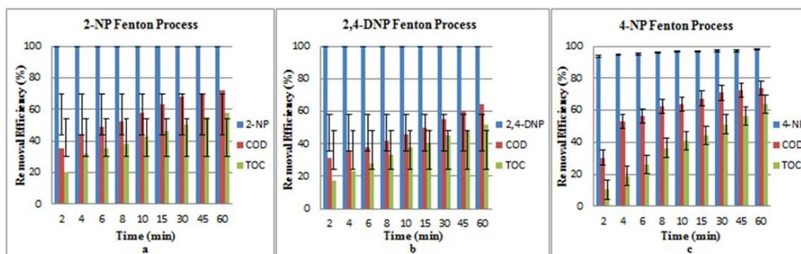
Fig. 3: Removal efficiencies for Fenton process (optimum conditions)
