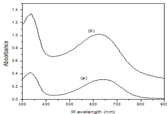
Fig. 3: UV-Vis spectra of (a) PANI-DBSA salt and (b) PANI-TiO<sub>2</sub> composite recorded in *N*-methylpyrrolidinone solution
