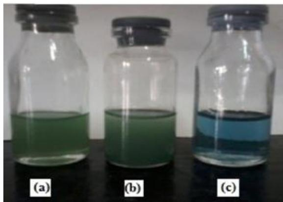
Fig. 2: Solution of PANI-TiO<sub>2</sub> composite in (a) chloroform, (b) 2:1 mixture of toluene + 2-propanol, and (c) DMSO.
