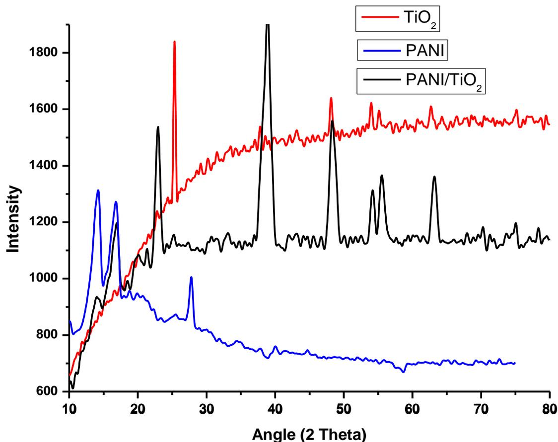
Fig. 5: XRD patterns of  $\text{TiO}_2$ , PANI and PANI-  $\text{TiO}_2$  composite.
