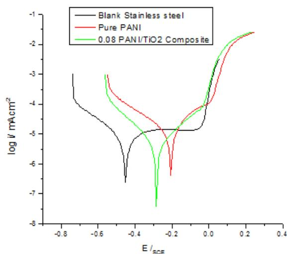
Fig. 9: The Tafel plots of uncoated, PANI and PANI-TiO<sub>2</sub> coated steel electrodes.
