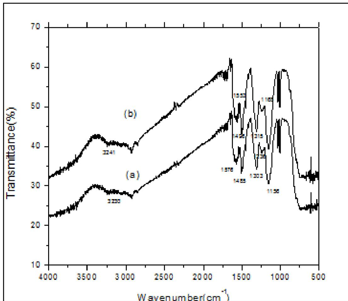
Fig. 6: FTIR spectra of (a) PANI powder and (b) PANI-TiO<sub>2</sub> composite.
