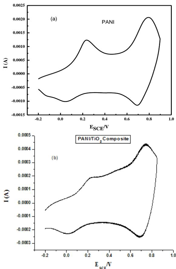
Fig. 8: CVs of (a) PANI and (b) PANI/TiO<sub>2</sub> composite on a gold sheet electrode, in 0.5 M H<sub>2</sub>SO<sub>4</sub> at a scan rate of 50 mV/s.
