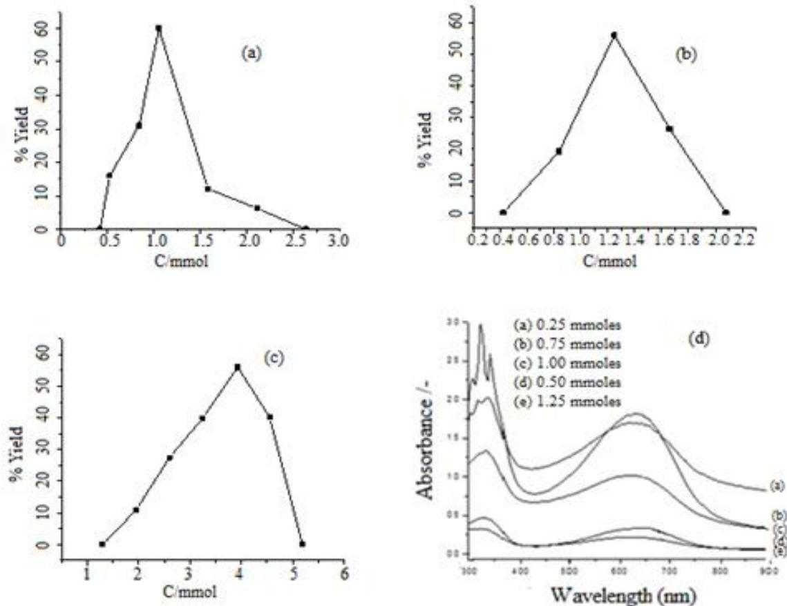
Fig. 1: Effect of a) monomer b) oxidant c) DBSA concentration on % yield and d) UV-Vis spectra of synthesized composites with different concentration of  $\text{TiO}_2$ .
