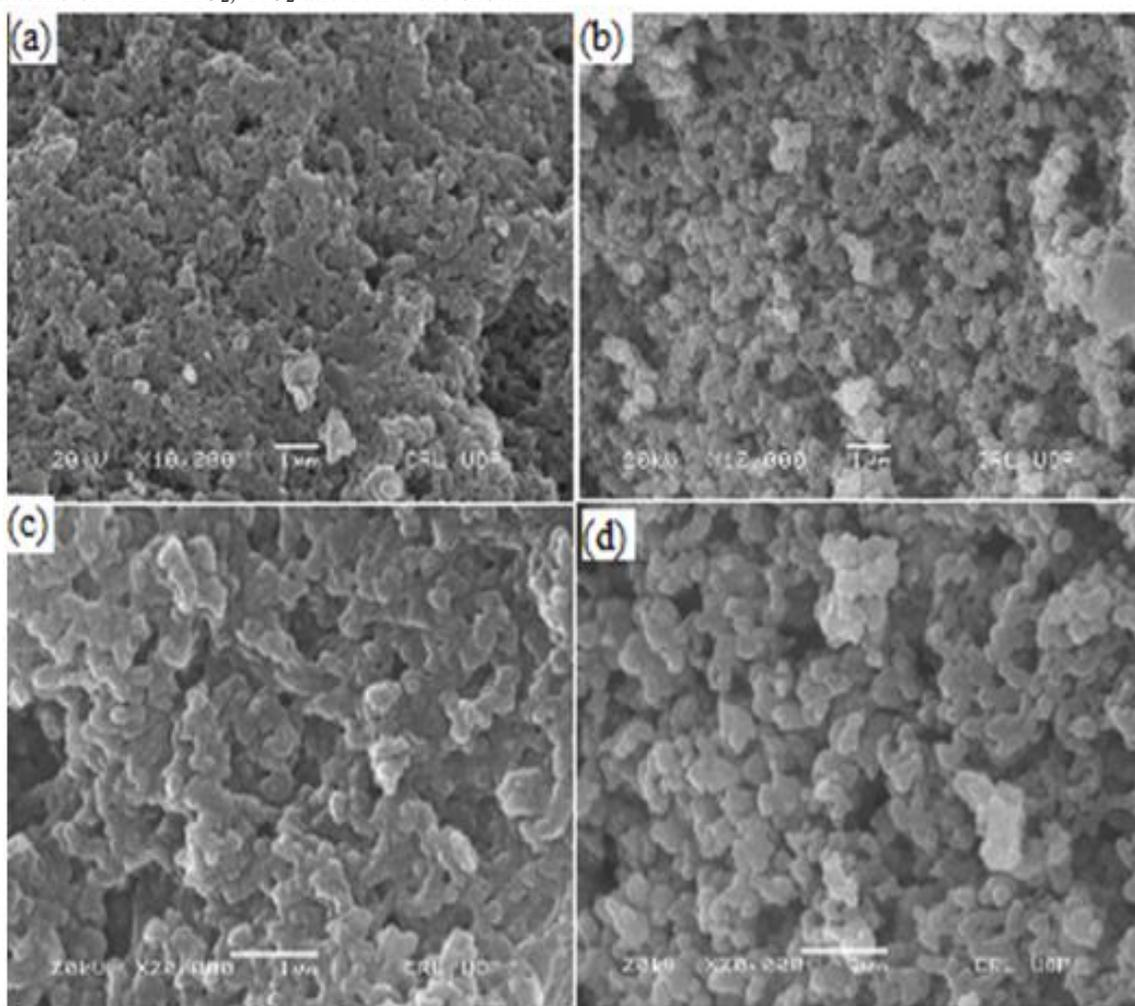
Fig. 4: (a). SEM images of PANI, (b) PANI- TiO<sub>2</sub> composite at lowmagnification , (c) SEM images of PANI and(d) of PANI- TiO<sub>2</sub> composite at high magnification.
