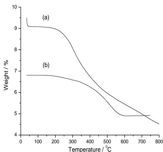
Fig.7: Thermogravimetric curves of (a) PANI and (b) PANI-TiO<sub>2</sub> composite.
