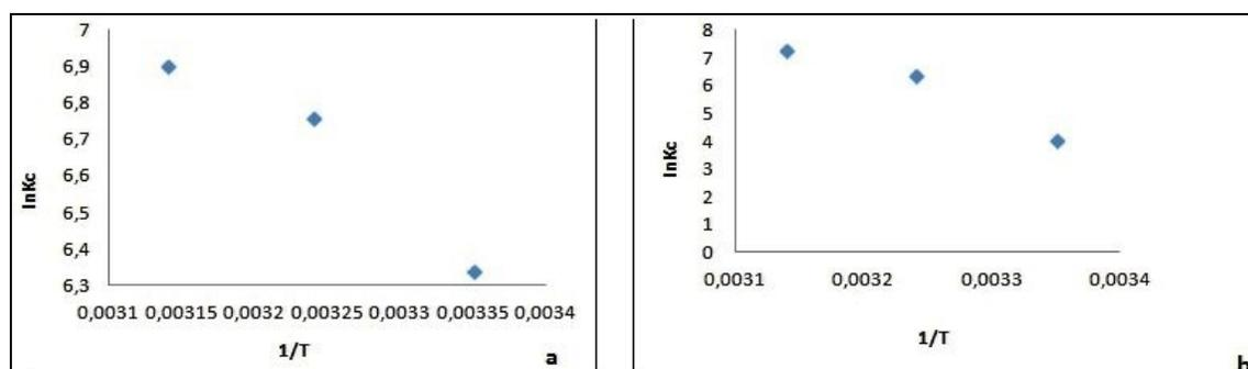
Fig. 8: (a). Clausius-Clapeyron equation for the adsorption of natural red with diatomite ( $C_0 = 20 \text{ mg/L}$ ,  $\text{pH} = 6.9$ ) and (b). Clausius-Clapeyron equation for basic blue adsorption with diatomite ( $C_0 = 20 \text{ mg/L}$ ,  $\text{pH} = 6.0$ ).
