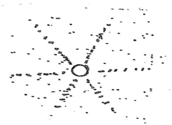
Fig. 13: Asterism in a Laue back-reflection photograph. The reflections from distorted or curved planes form elongated spots. [7].
