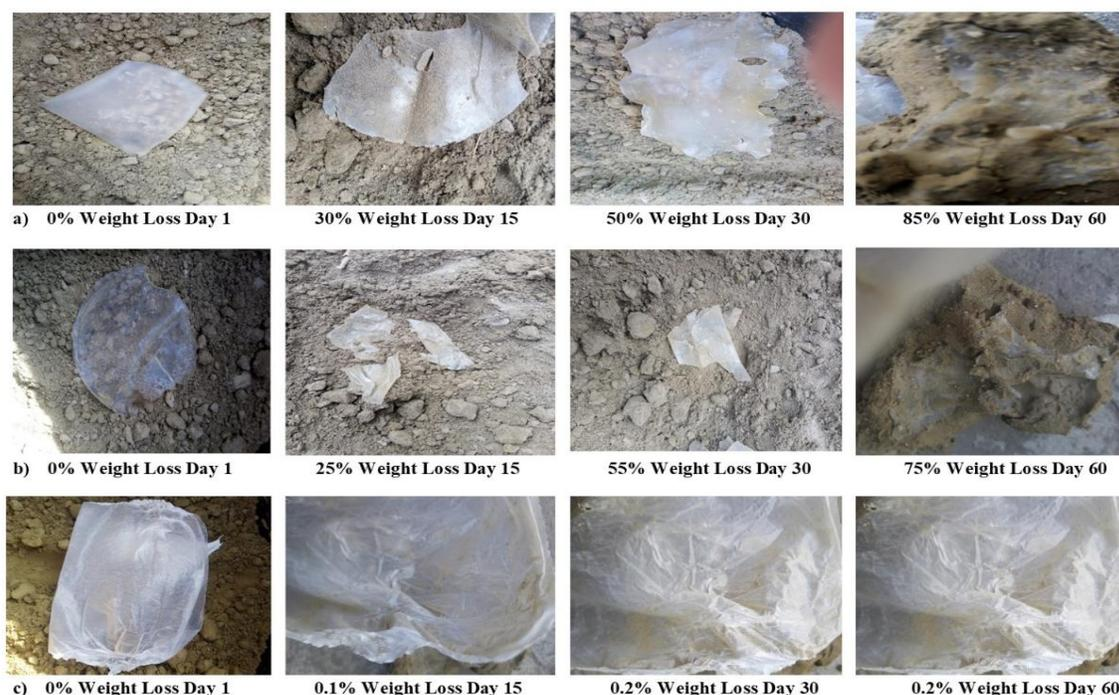
Fig. 8: Biodegradation of (a) starch bioplastic, (b) 5% ZnO NPs reinforced composite bioplastic, and (c) polyethylene plastic.
