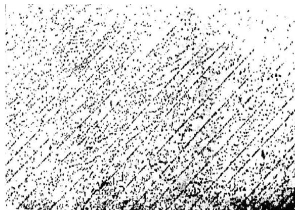
Fig. 11: Bent, annealed and etched single crystal of aluminium, showing sub-boundaries. X70 (After Cahn {1949}). [13]
