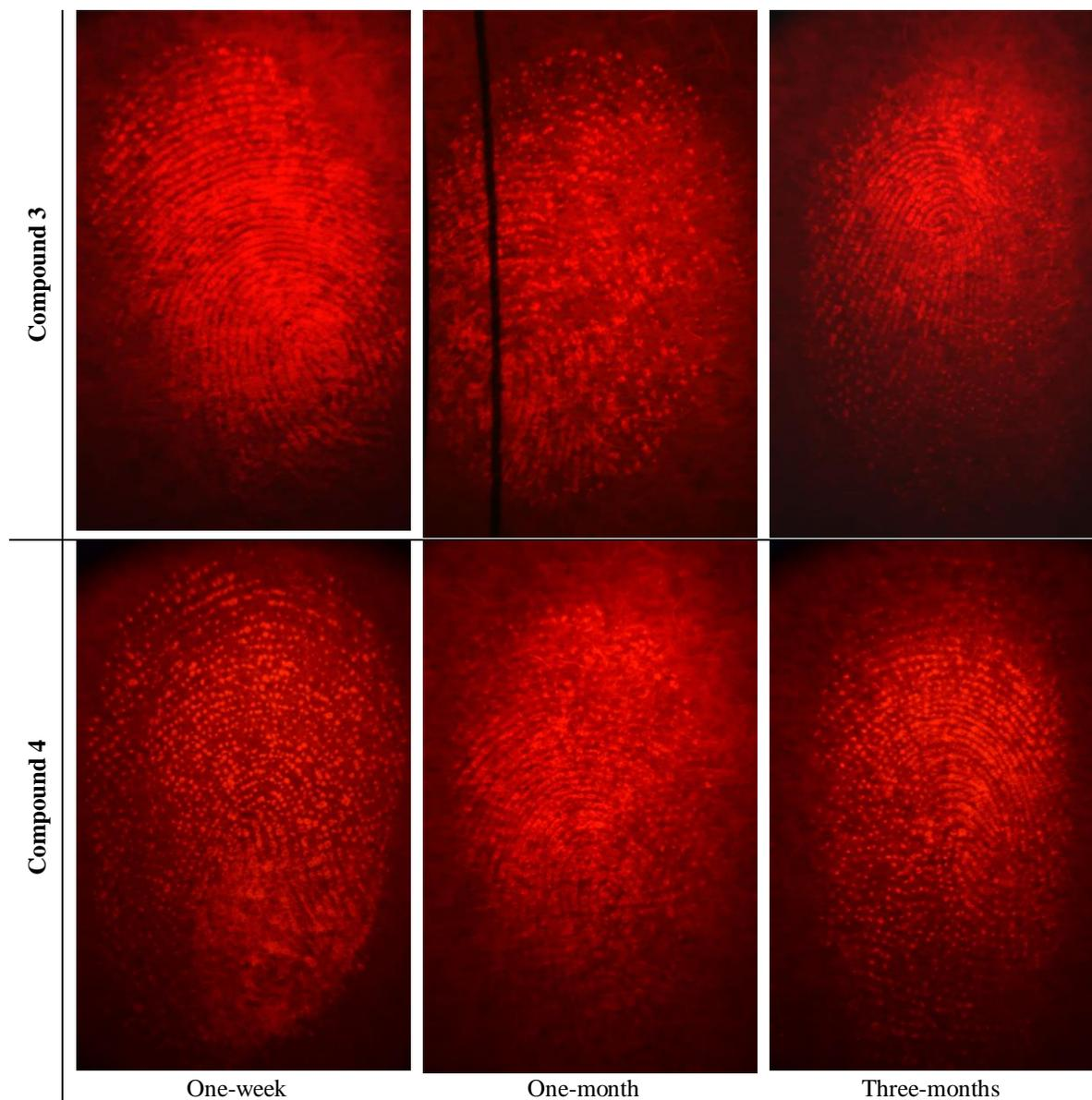
Fig. 6: Aged latent fingerprints developed with phenothiazines **3** and **4**.
