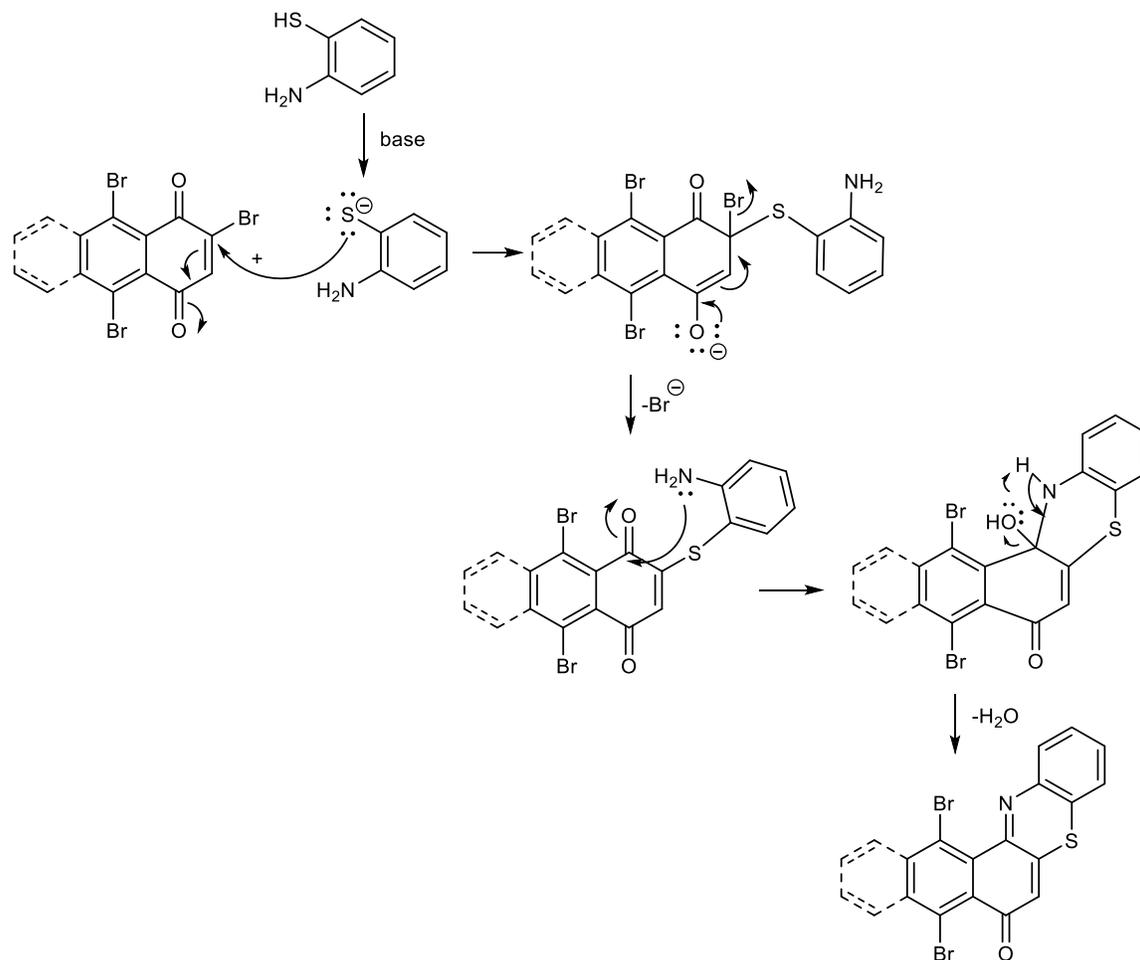
Fig. 3: The reaction mechanism for the formation of the **3** and **4**.
