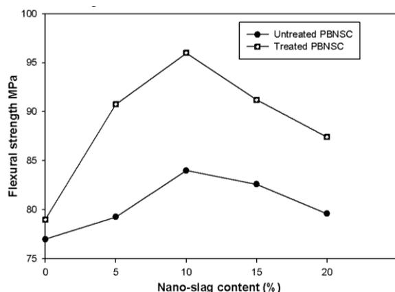
Fig. 2: Effect of nano-slag content on the flexural strength values of both untreated and treated particleboard composites (PBNSC).
