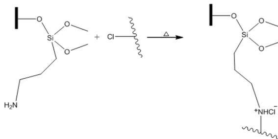
Scheme-1: Interaction between treated rice husk fiber and polyvinyl chloride.
