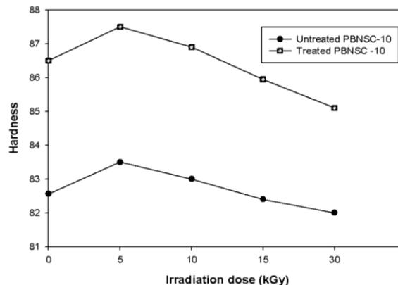
Fig. 5: Effect of gamma-irradiation doses on the hardness values of both untreated and treated particleboard composites containing 10% nano-slag (PBNSC-10).
