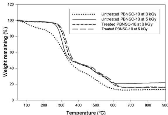
Fig. 8: TGA thermograms of both untreated and treated particleboard composites containing 10% nano-slag (PBNSC-10) at 0 and 5 kGy of gamma rays.
