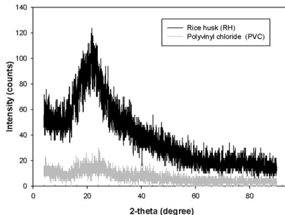
Fig. 10: XRD diffraction of both rice husk fiber (RH) and polyvinyl chloride (PVC).
