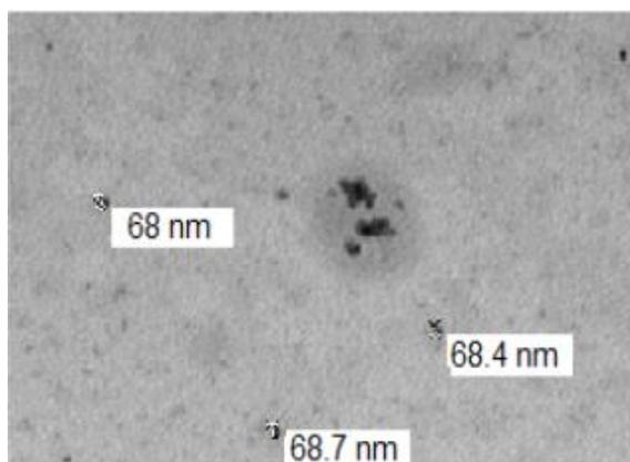
Fig. 1: Transmission electron microscopy of nano-slag.
