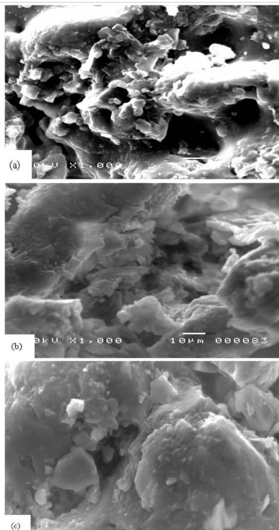
Fig. 12: SEM micrographs for (a) untreated particleboard composite (PBNSC-10) at 0 kGy, (b) treated particleboard composites (PBNSC-10) at 0 kGy (c) treated particleboard composites (PBNSC-10) at a dose of 5 kGy.
