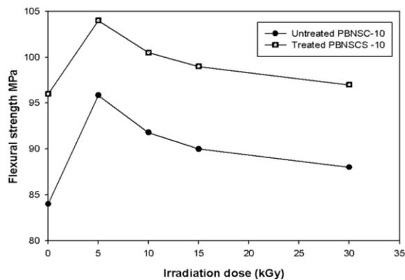
Fig. 3: Effect of gamma-irradiation doses on flexural strength values of both untreated and treated particleboard composites containing 10% nano-slag (PBNSC-10).
