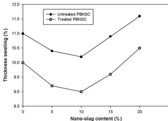
Fig. 6: Effect of nano-slag content on the thickness swelling percentage of both untreated and treated particleboard composites (PBNSC).
