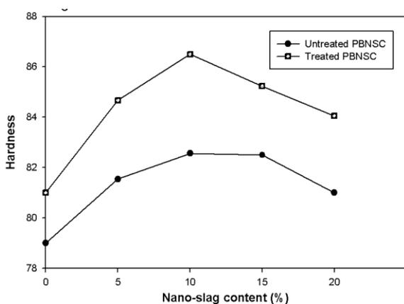
Fig. 4: Effect of nano-slag content on the hardness values of both untreated and treated particleboard composites (PBNSC).
