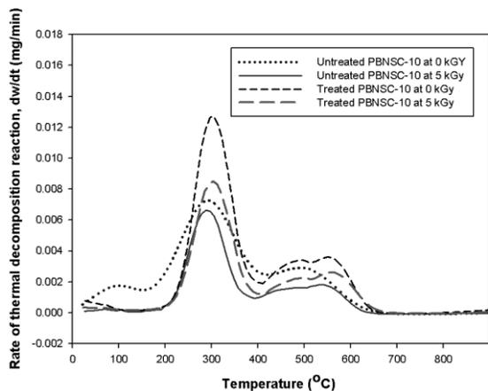
Fig. 9: Rate of thermal decomposition reaction (dw/dt) of both untreated and treated particleboard composites containing 10% nano-slag (PBNSC-10) at 0 and 5 kGy of gamma rays.
