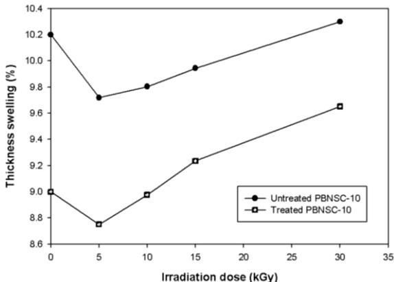
Fig. 7: Effect of gamma-irradiation doses on the thickness swelling percentage of both untreated and treated particleboard composites containing 10% nano-slag (PBNSC-10).
