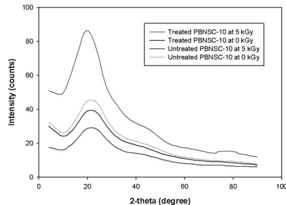
Fig. 11: XRD diffraction of untreated and treated particleboard composites containing 10% nano-slag (PBNSC-10) at 0 kGy and 5 kGy.
