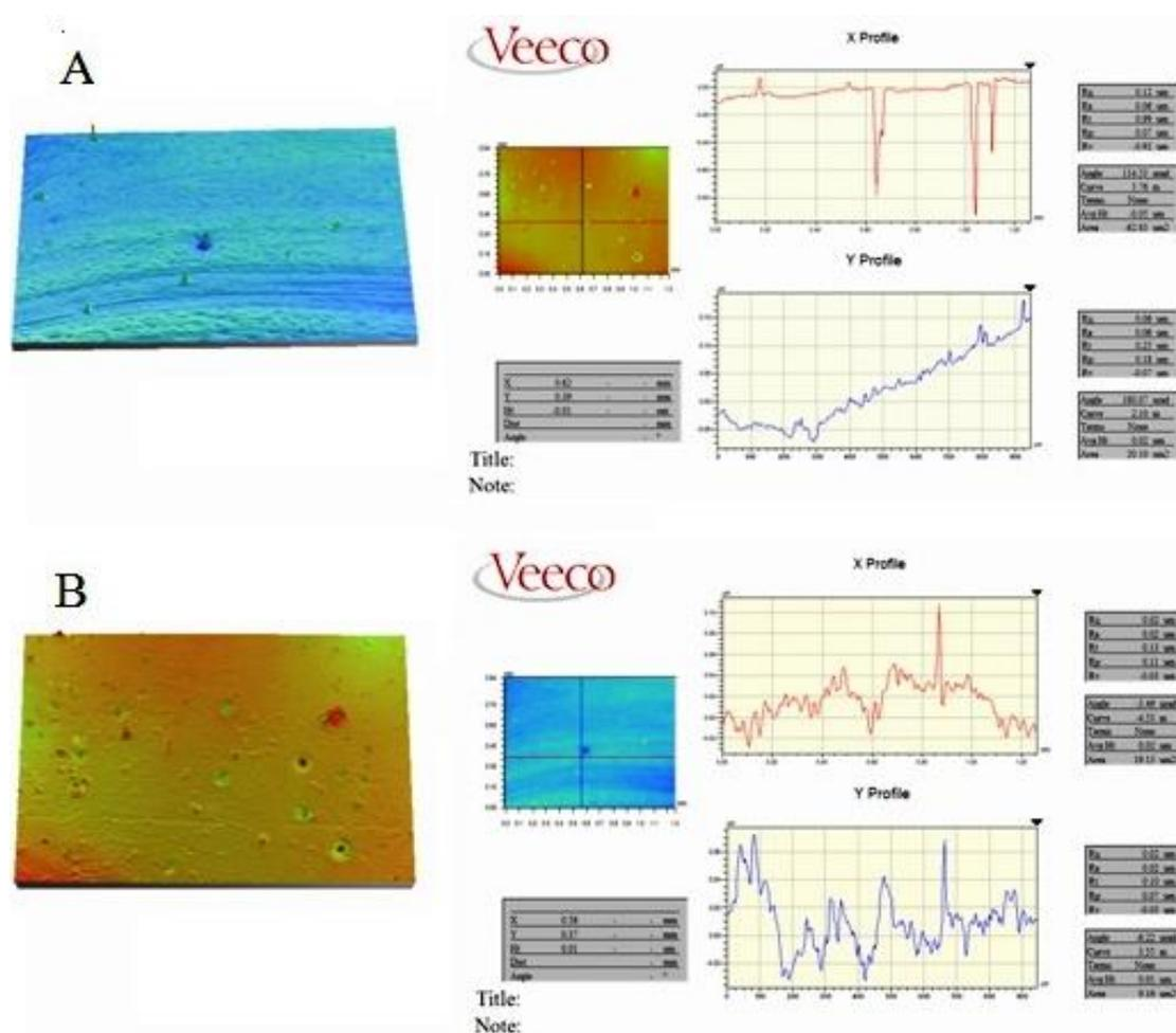
Fig. 1: Optical profilometer images (0.9 x 1.3 mm) and side profiles for whey protein gels deposited on untreated glass surface A: 20 mM Ca<sup>2+</sup>, B: 30mM Ca<sup>2+</sup>.
