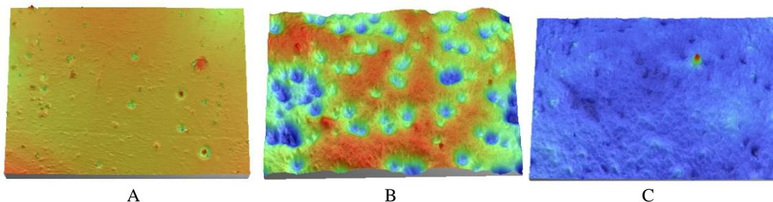
Fig. 2: Optical profilometer images (47 x 62  $\mu\text{m}$ ) for whey protein gels induced by 30 mM  $\text{Ca}^{2+}$  deposited on: A - untreated glass surface, B - Ar plasma activated glass and C - air plasma activated glass.
